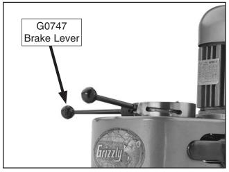
Figure 39. Model G0747 brake lever.
